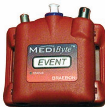
Fig. 8. Braebon Medibyte, a miniature 10-channel PSG diagnostic screener.
